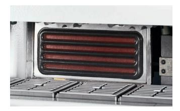
Workpiece preheating with heaters
